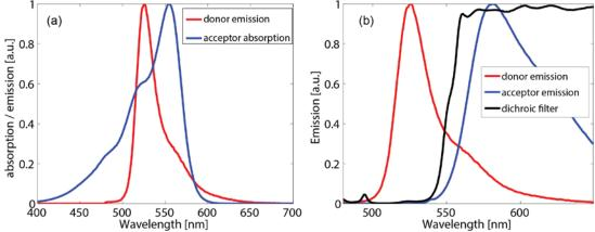
Fig. 1: (a) Overlap of donor (mAmetrine) emission and acceptor (tdTomato) absorption spectrum. (b) Donor and acceptor emission spectra superimposed with transmission profile of the dichroic filter that separates the collected fluorescence into the two detection channels
